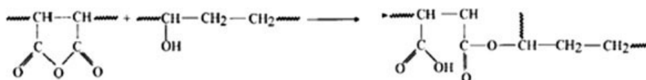
Scheme 1 Potential reaction between the carbonyl groups of MAH and hydroxyl group of EVOH.
